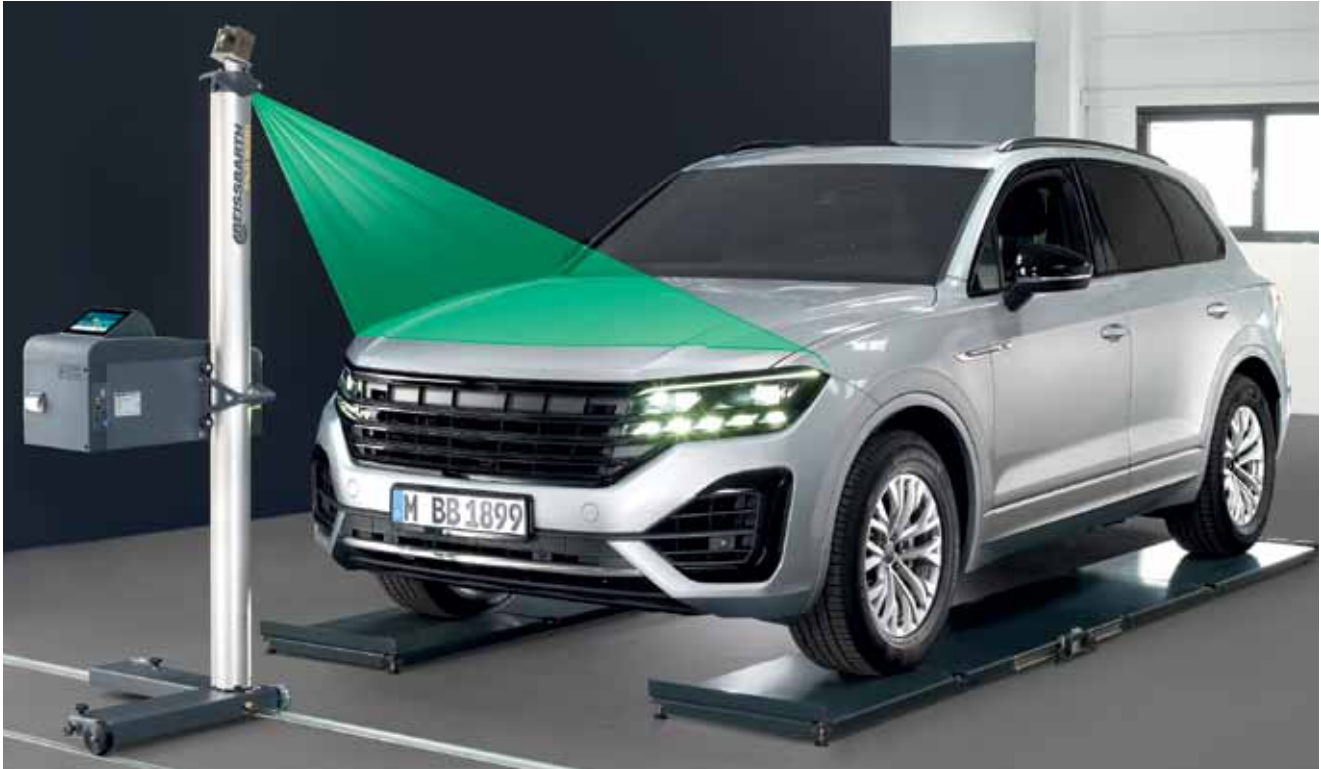
Adjustment of a headlight on rail system, combined with LTB 100 leveled test bay
