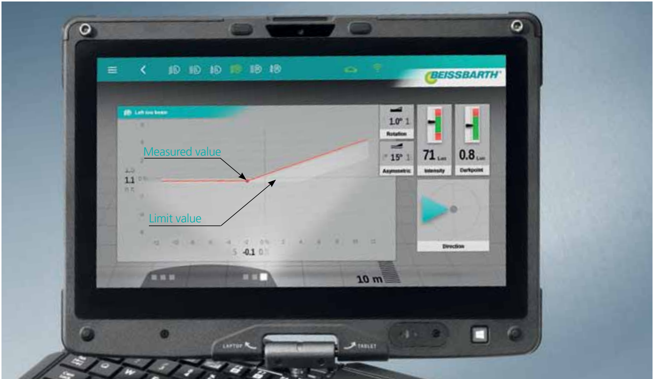
Accurate display of the test results on the workshop computer
