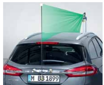
Green vertical laser for symmetrical axis alignment as optional accessory
