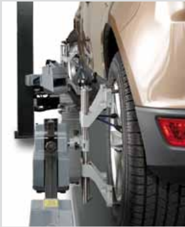
Easy CCD: CCD wheel alignment
