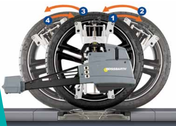
Rolling runout compensation (Easy CCD)
